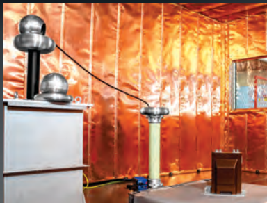
PARTIAL DISCHARGE TEST
