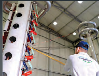
LIGHTNING IMPULSE VOLTAGE TEST
